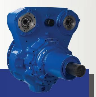
The HPTO15 is a hydraulically applied wet friction clutch designed for off-highway diesel engine driven equipment. Its hydraulic design eliminates the need to adjust the clutch throughout its wear life. The HPTO15 can be combined with either of PT Tech's existing pump drive housings, the FX Housing (4 pump pads) or VG Housing (2 pump pads).
