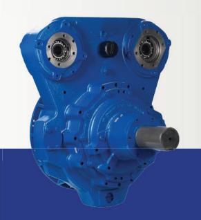
The HPTO14 is a hydraulically applied wet friction clutch designed for off-highway diesel engine driven equipment. Its hydraulic design eliminates the need to adjust the clutch throughout its wear life. The HPTO14 can be combined with either of PT Tech's existing pump drive housings, the FX Housing (4 pump pads) or VG Housing (2 pump pads).
