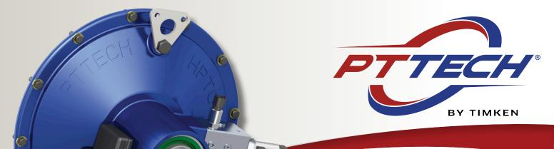
The HPTO8 is a hydraulically applied clutch. It's friction plates operate in a dry environment. It's hydraulic design eliminates the need to adjust the clutch throughout its wear life.
